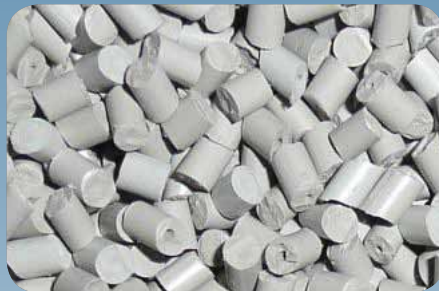
CELLIANT MASTER BATCH made from liquid PET and Celliant powder
